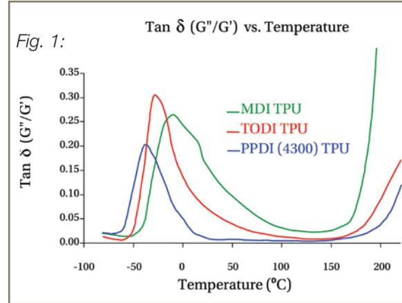
Resilon's internal heat build-up (hysteresis) is much lower across the entire temperature range of operation (-40° to +275°F)
